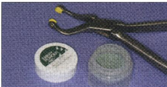
Figure 5. GC pliers have replaceable rubber grips at beak end. Emery powder may be used for additional friction.
